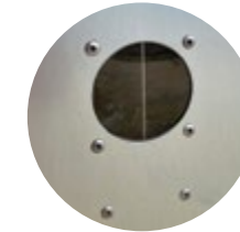
Division sheet in the hopper allows 2 feeds to be used
