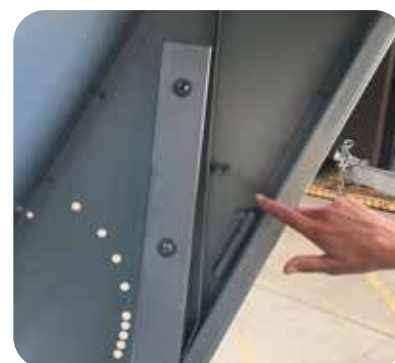
IMAGE: FEEDER CLEANING TOOL AND TUBE SPANNER STORAGE LOCATION
