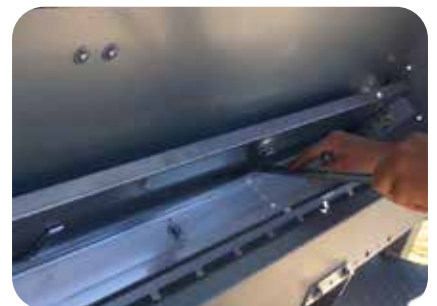
Cleaning the feed access area
