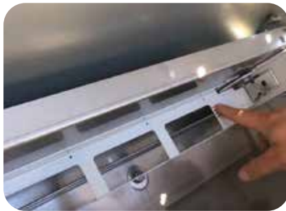
Inverting the Adjuster Guard
