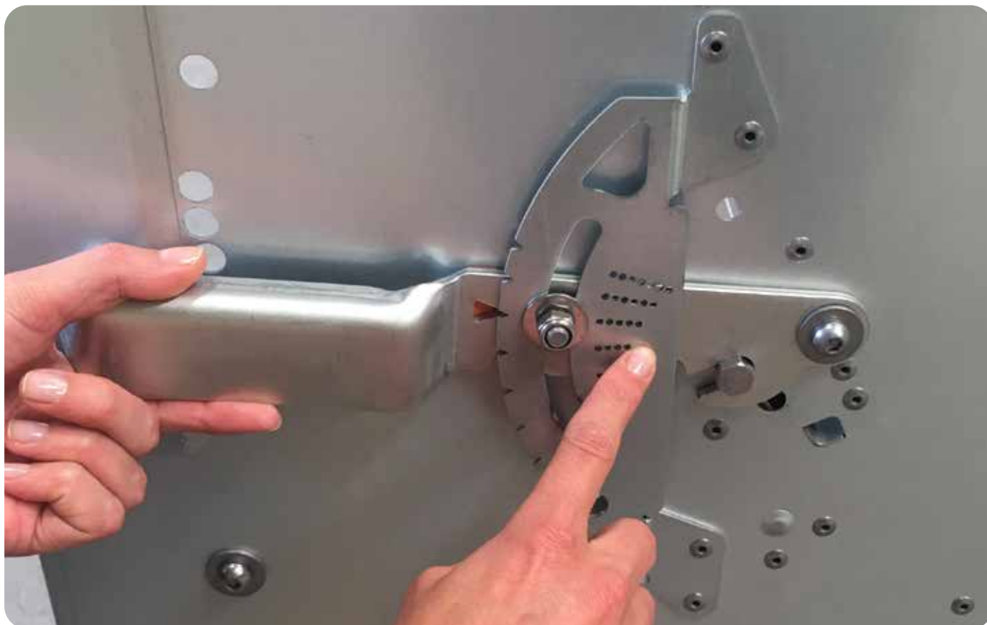
ABOVE IMAGE: USE THE UPPER ADJUSTER HANDLES TO SET THE UPPER ADJUSTER
